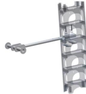
The tube and clamp assembly is designed to tie the P.U. from the mast to the building wall, floor or ceiling, allowing passage through openings such as windows, doors etc... The tube clamps and tubes are not provided by Bennu. We recommend the use of tubes of 2" diameter and standard 2" tube clamps.
