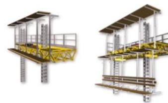
*Install 6' outriggers in top multi-function bracket pockets, making sure not to extend more than 48" from the center of the multi-function bracket to the end of outrigger and secure with 5/8" bolts, using a 15/16" wrench.*
