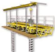
*Install 6' outriggers in top multi-function bracket pockets and secure with 5/8" bolts, using 15/16" wrench.*
